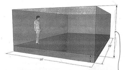
169. Calculate the volume of concrete in the floor of the 7 starts aquarium in cubic feet.
